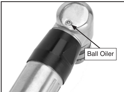
Figure 4. Ball oiler location.
