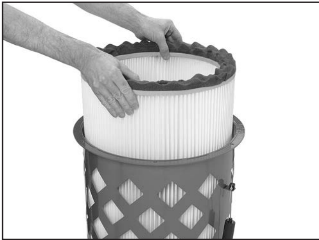
Figure 65. Removing the filter from the canister assembly.
