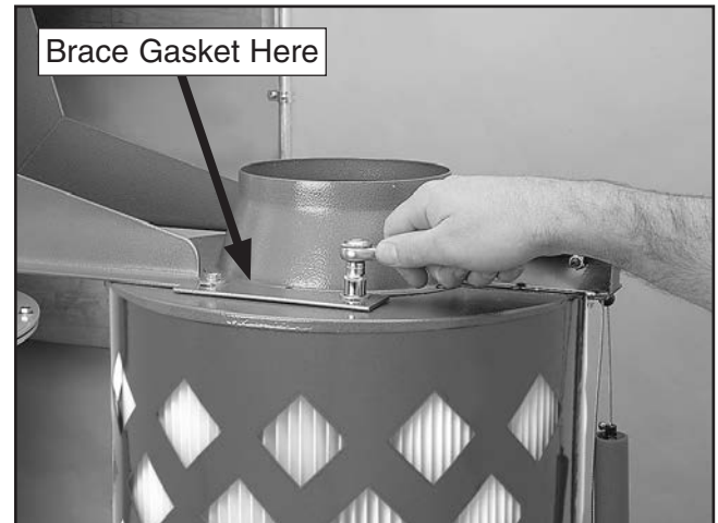
Figure 19. Mounting filters to the braces.
