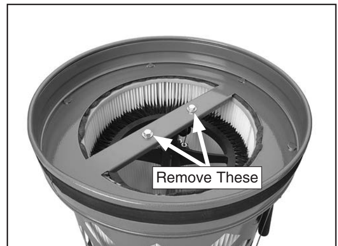
Figure 64. Cross support fasteners.
