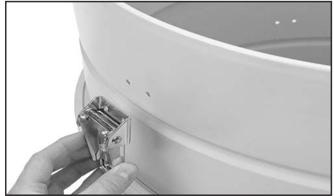
Figure 26. Installing drum latches on collector drum.
