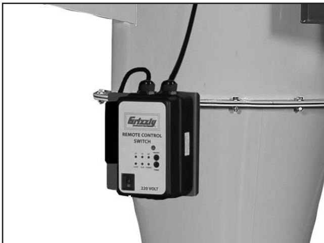
Figure 33. Switch mounted to funnel.
