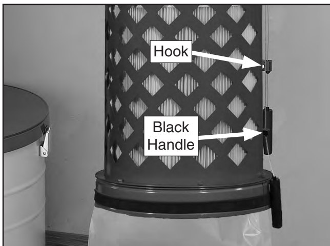
Figure 59. Black handle cable secured in the handle hook.
