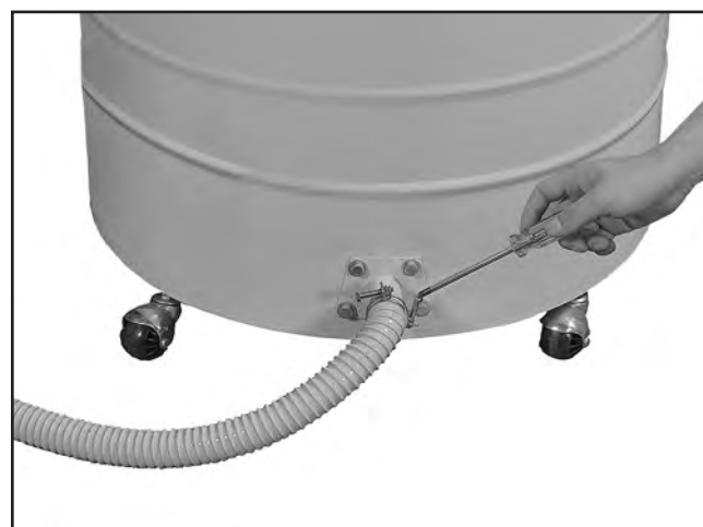
Figure 29. Connecting the vacuum hose.
