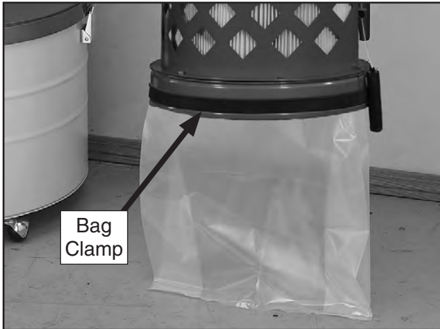
Figure 30. Plastic collection bag clamped in place under filter.
