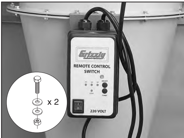
Figure 31. Magnetic switch mounted to funnel.
