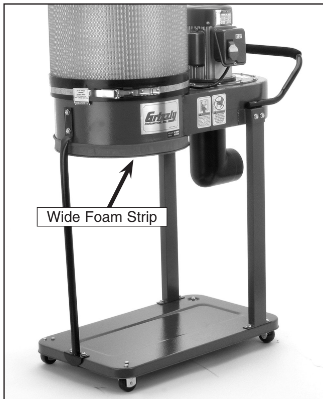
Figure 12. Installed and trimmed wide foam strip.
