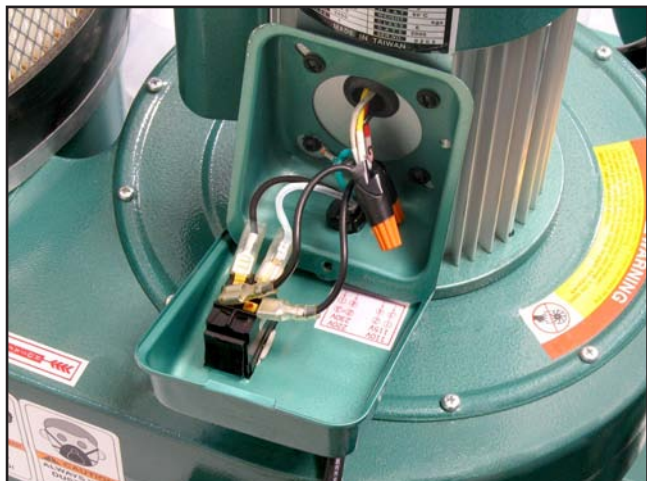
Figure 21. Motor junction box wiring.
