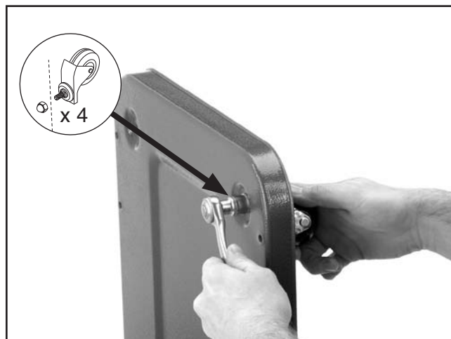
Figure 6. Caster installed onto the base.
