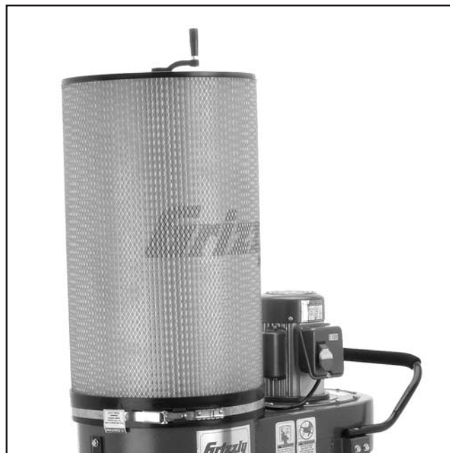
Figure 11. Canister filter installed and secured.
