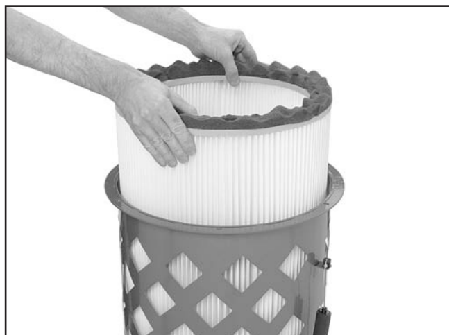
Figure 92. Removing the filter from the canister assembly.
