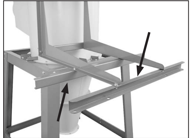
Figure 33. Long brace supports attached.
