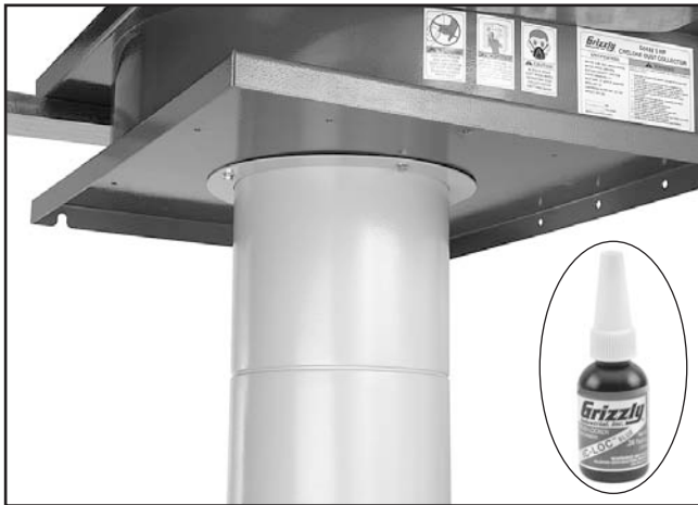
Figure 21. Intake cylinder mounted to blower housing.
