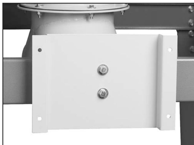
Figure 49. Model G0638 control box bracket mounted.
