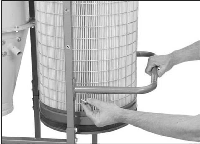
Figure 11. Installing the hand rail.
