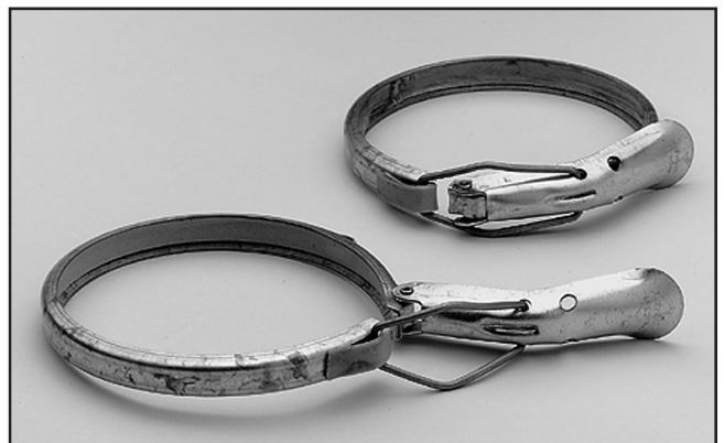
Figure 34. Dust collection pipe clamps.
