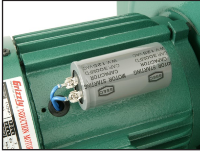
Figure 40. Start Capacitor. 110 Volt Motor
