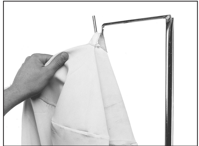
Figure 11. Attaching upper filter bag.
