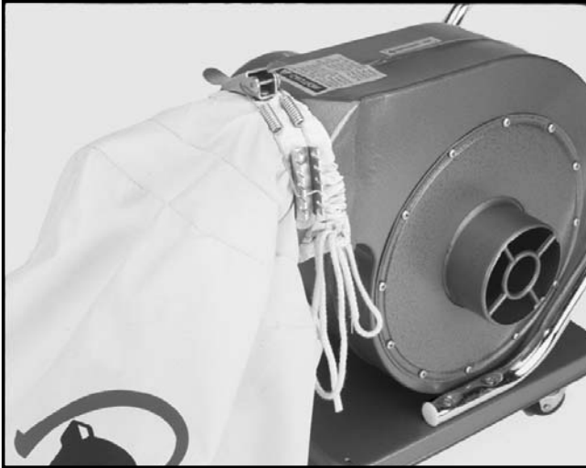
Figure 5. Bag clamped to the outlet end of the collector body.
