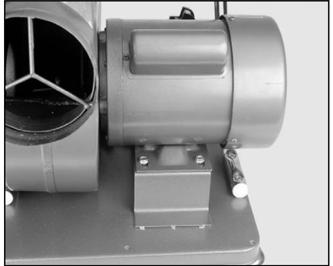
Figure 4. Motor/collector body mounted on base.
