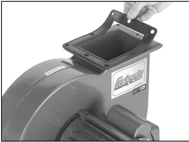
Figure 9. Placing rubber gaskets over outlet.
