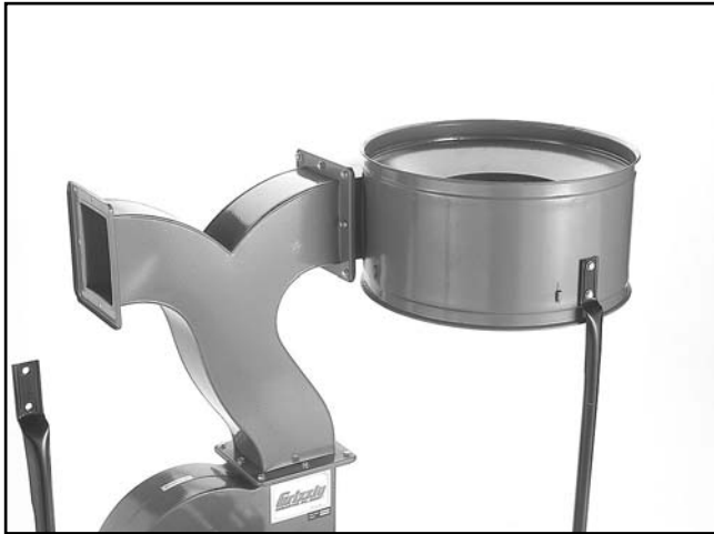
Figure 12. Collector ring installed.
