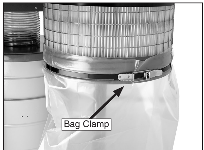
Figure 30. Canister filter collection bag installed.
