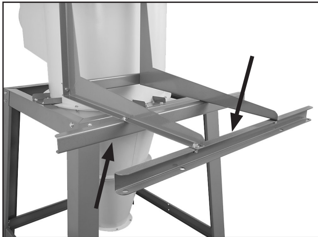
Figure 27. Long brace supports attached.
