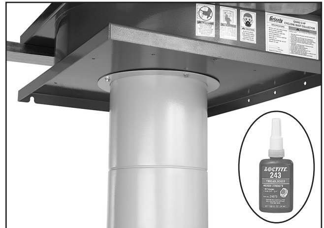
Figure 16. Intake cylinder mounted to blower housing.
