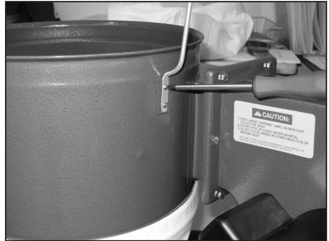
Figure 10. Installing upper bag support.
