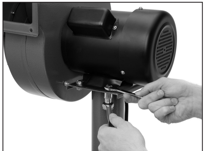
Figure 7. Installing motor/impeller housing on collector support.
