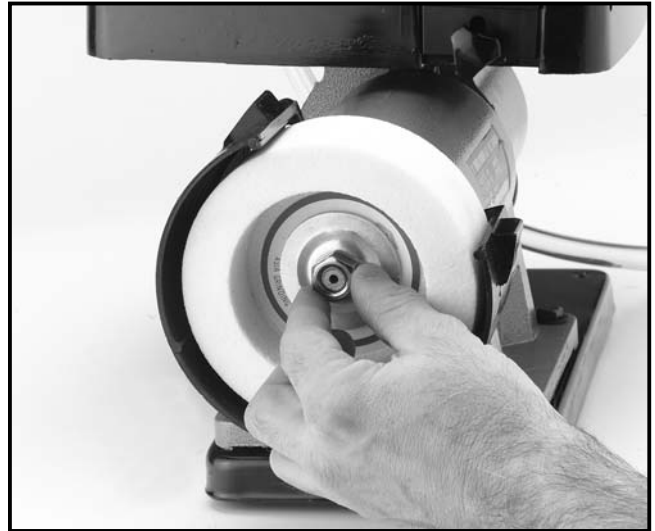
Figure 10. Removing dry wheel.
