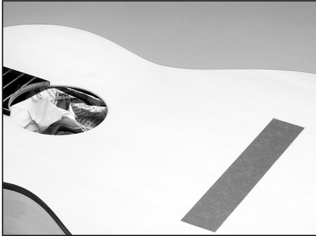
Figure 8. Masked bridge area and blocked sound hole.
