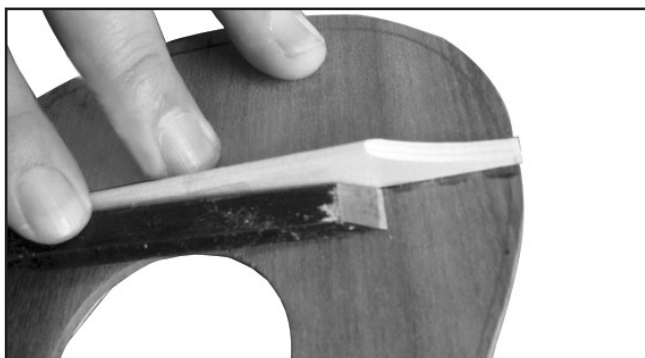
Figure 14. Example of scraping glue squeezed-out while still soft.
