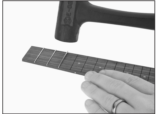
Figure 23. Installing the frets.
