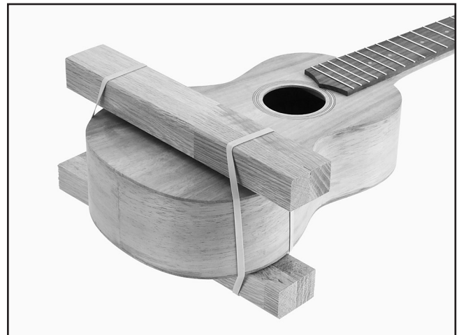
Figure 31. Gluing the bridge to the body.
