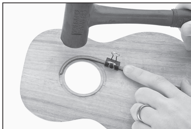
Figure 8. Installing the purfling.
