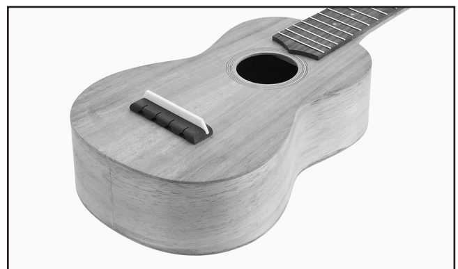
Figure 32. Bridge and saddle installed on the sound board.
