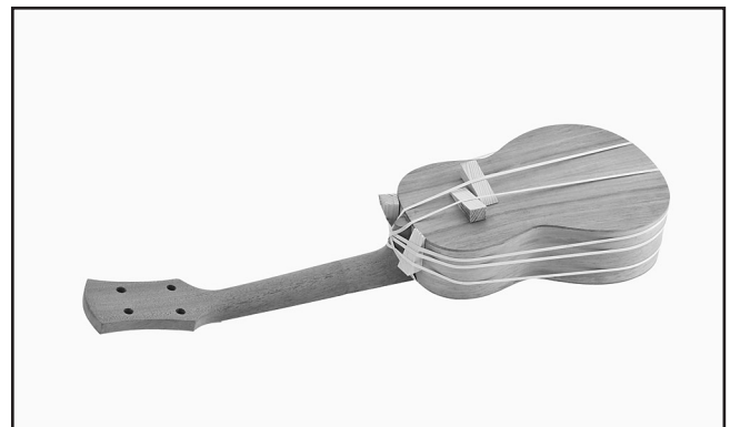
Figure 25. Gluing the neck to the body using rubber bands and wedges to secure it in place.
