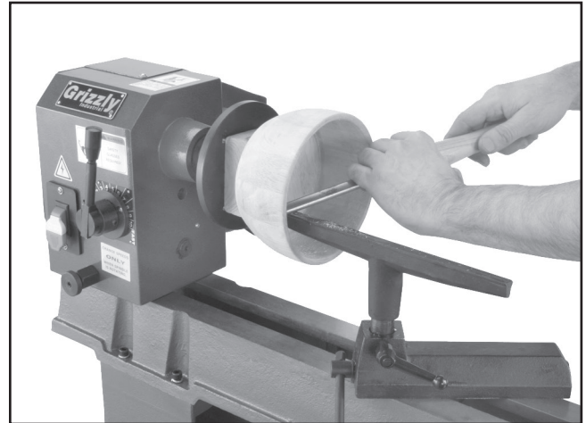
Figure 26. Typical faceplate turning operation.
