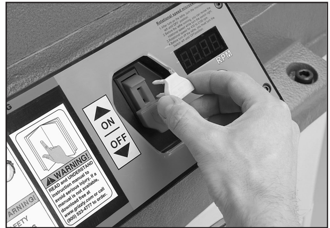
Figure 10. Removing safety key to disable the switch.
