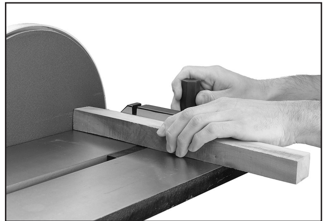
Figure 31. Typical disc sanding operation.
