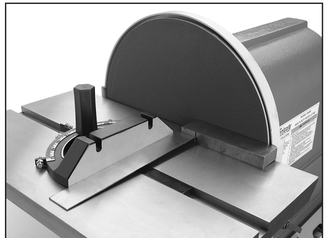
Figure 54. Squaring miter gauge to disc.
