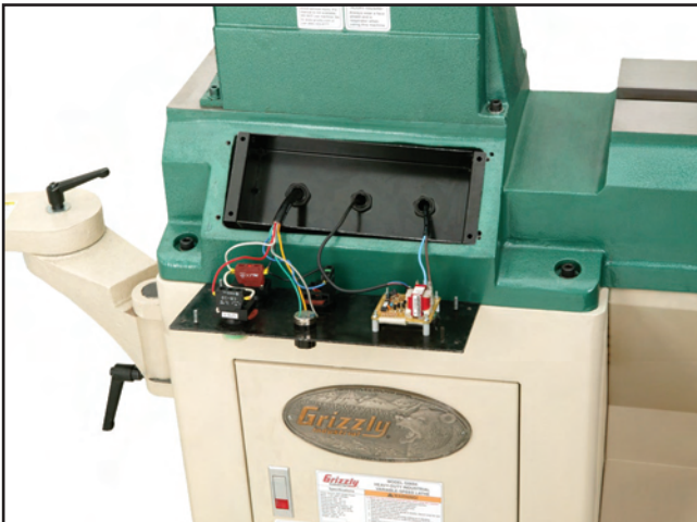
Figure 72. Control panel wiring.
