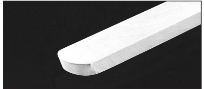
Figure 28. Example of a round nose scraper.
