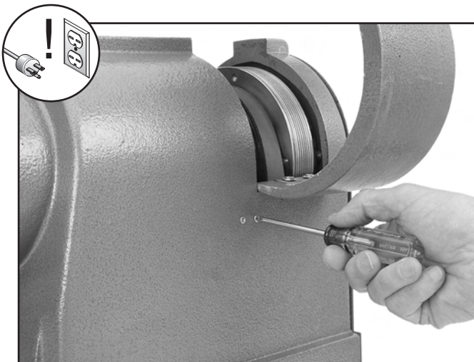
Figure 61. Removing speed sensor screws.
