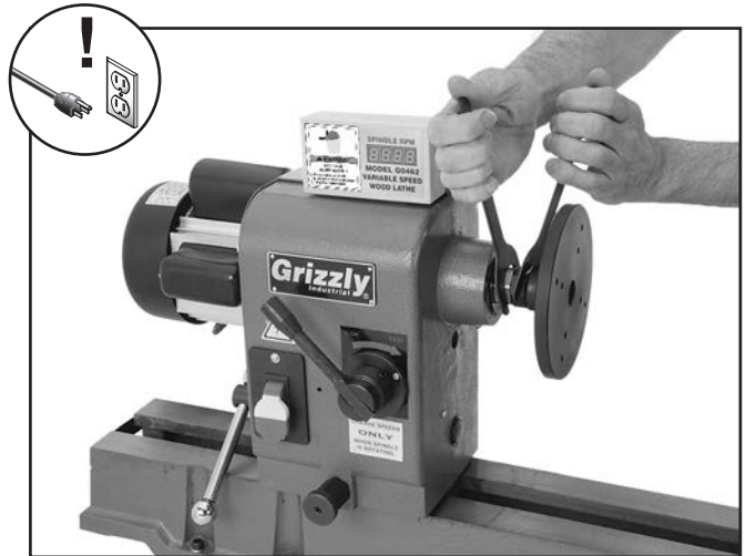
Figure 25. Tightening the faceplate onto the spindle.
