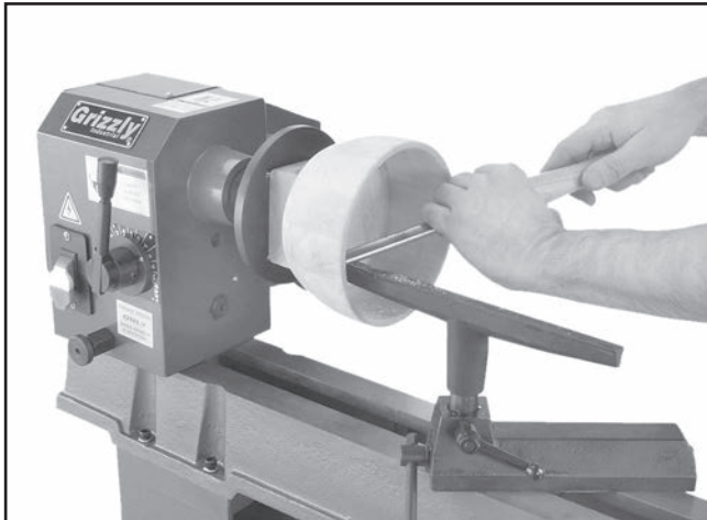
Figure 36. Typical faceplate turning operation.
