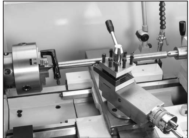
Figure 52. Example photo of stock mounted between the centers.
