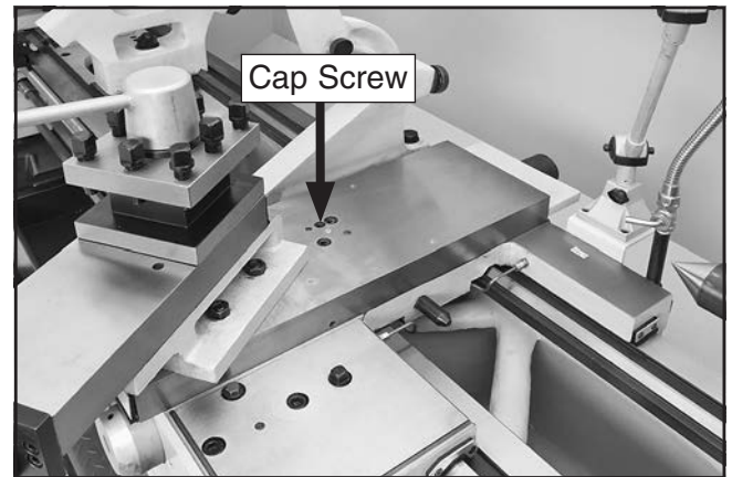
Figure 127. Cross slide backlash adjustment screw.
