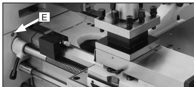
Figure 119. Leadscrew selection lever ball oiler.
