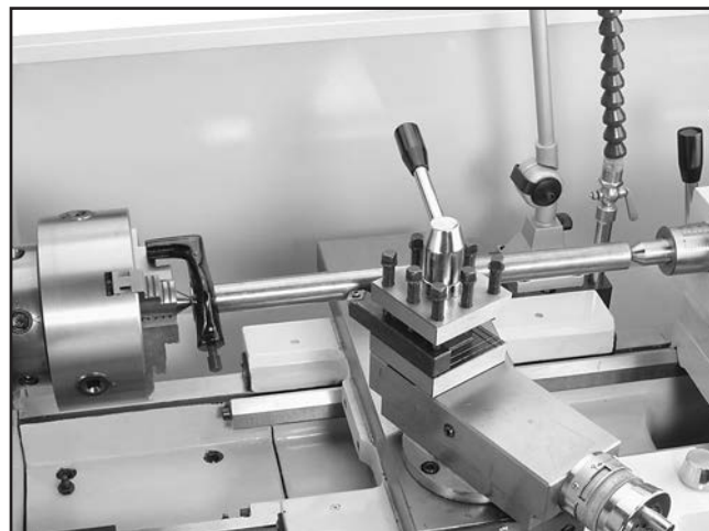
Figure 58. Example photo of a workpiece mounted between the centers.
