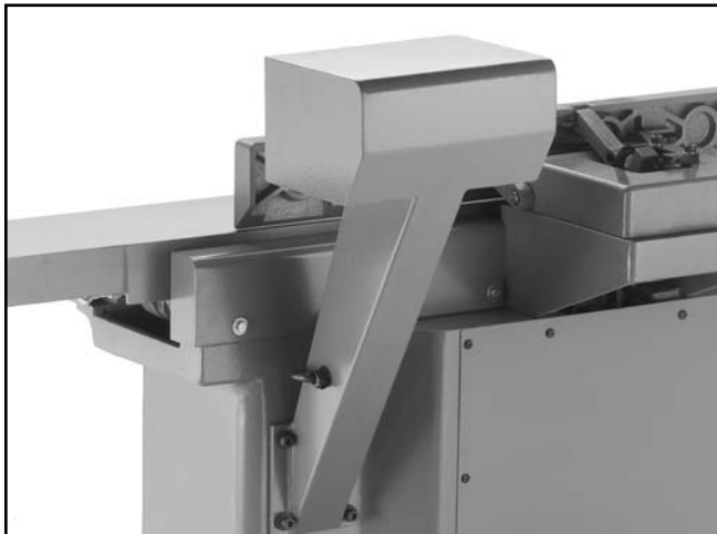
Figure 7B. Mounted pedestal switch.
