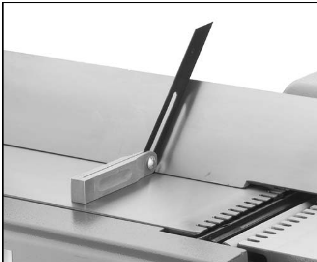
Figure 16. Using a 45° gauge to align fence.
