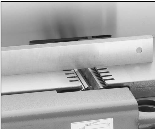
Figure 13. Setting the depth of cut scale.
