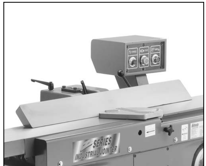
Figure 20. Fence position for bevel jointing.
