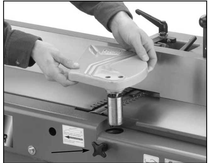
Figure 6a. Attaching cutterhead guard.
