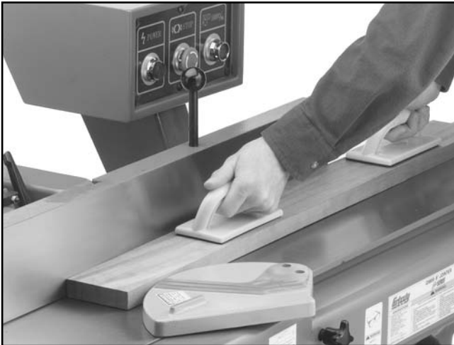
Figure 21. Correct method for surface planing.
