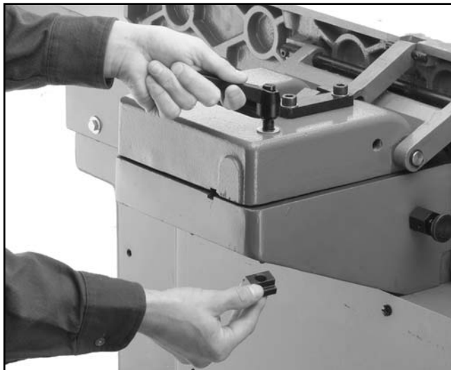
Figure 5. Fence base lock knob attachment.
