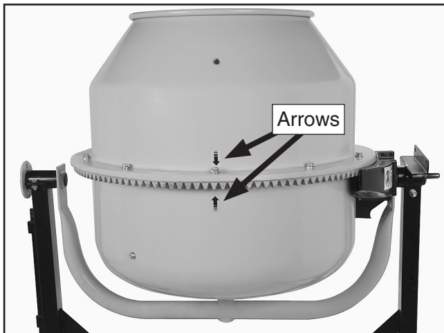
Figure 11. Upper drum attached to lower drum.
