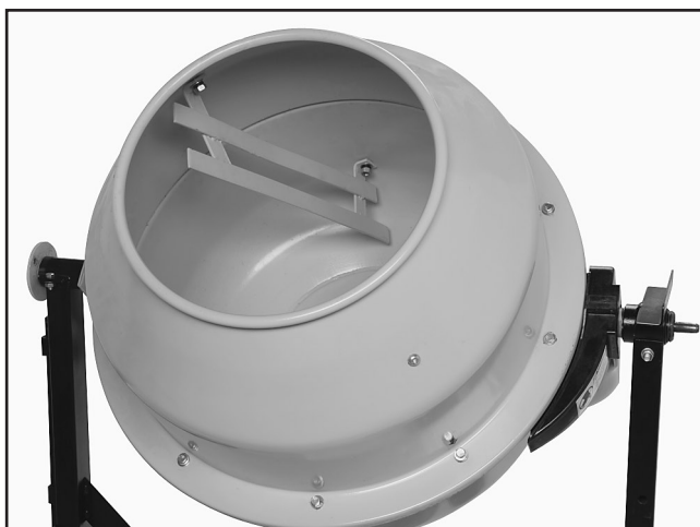
Figure 12. Upper part of mixing blades attached to upper drum.
