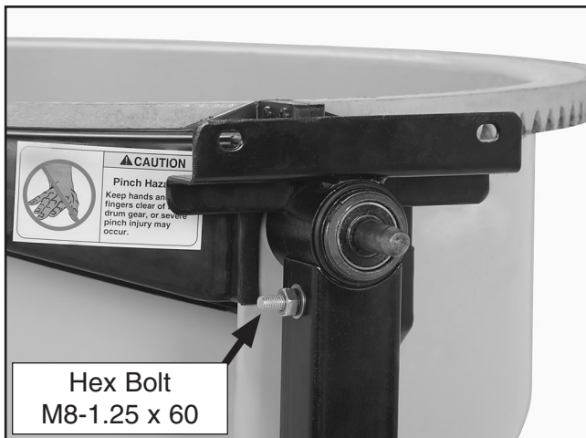
Figure 8. Bearing block installed over shaft and attached to frame.
