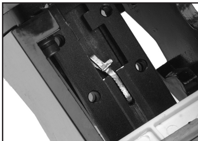
Figure 7. Jammed nail in discharge area.
