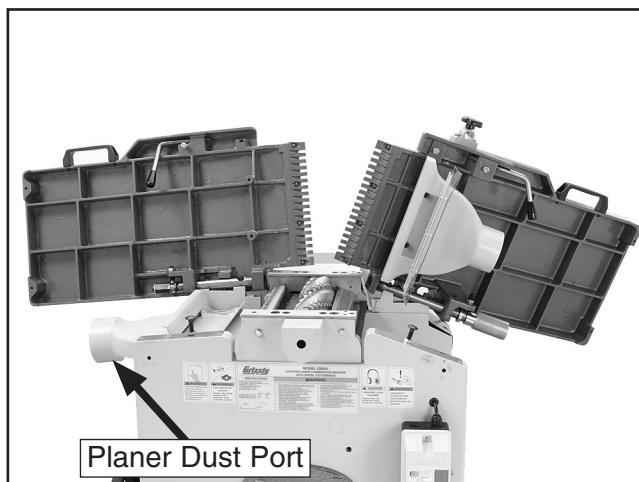
Figure 27. Planer dust port in "down" position.
