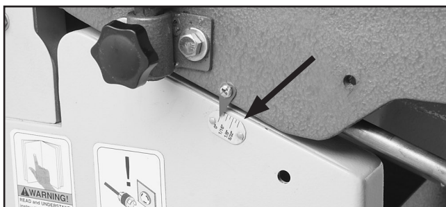
Figure 66. Depth scale adjusted to "0" position.
