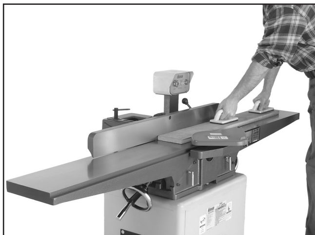
Figure 32. Typical surface planing operation.
