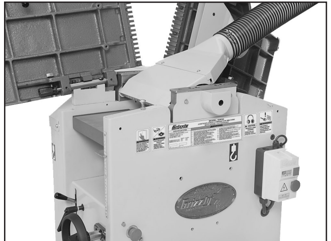
Figure 16. Dust hose attached to planer dust port.
