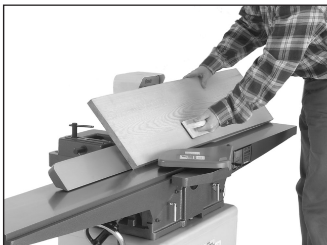
Figure 36. Typical bevel cutting operation.
