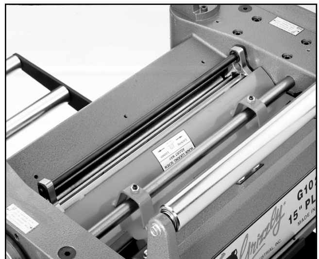
Figure 15. Cover Removed, Jig on cutterhead
