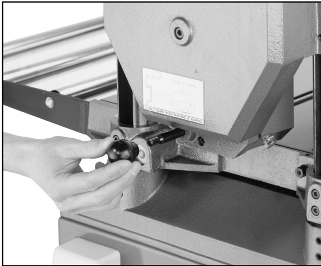
Figure 4. Installing speed change knob.
