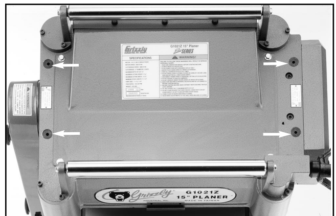
Figure 41. Feed roller lubrication points.
