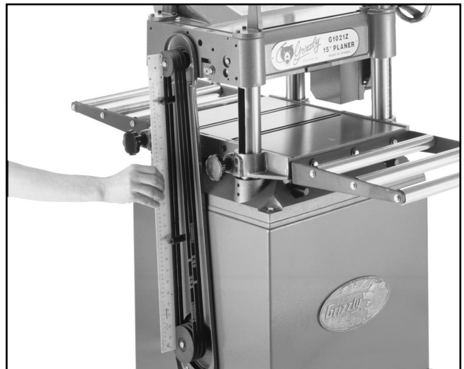
Figure 31. Checking pulley alignment.
