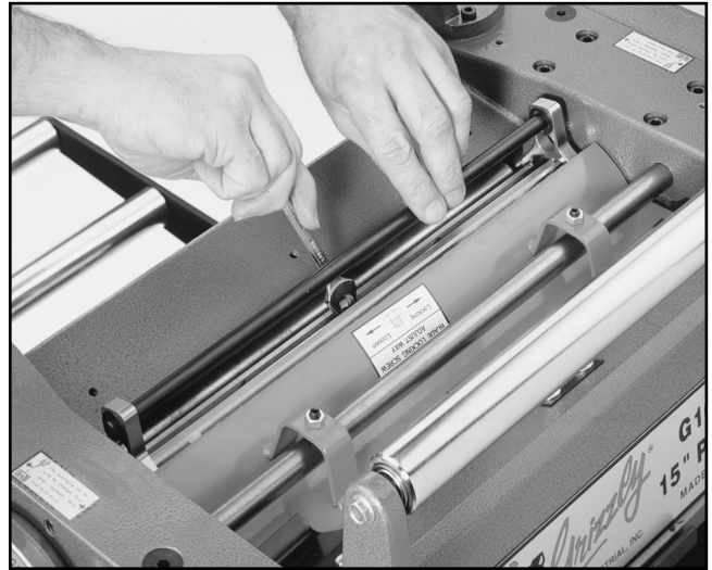
Figure 20. Tightening knives in cutterhead.
