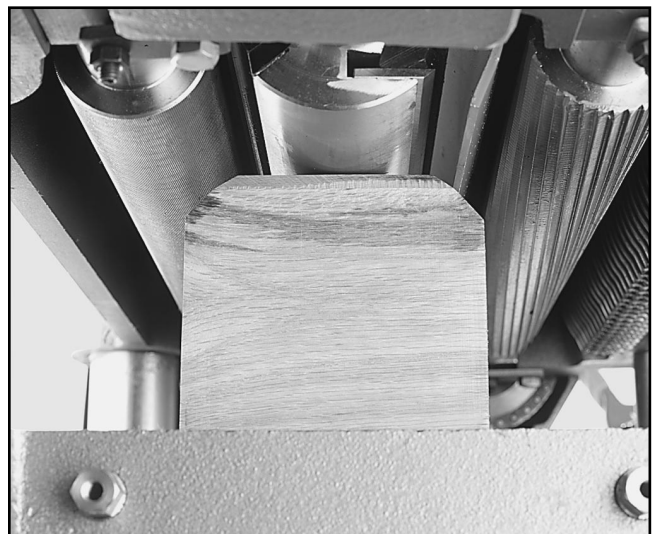
Figure 11. Guide block indicates parallelism.
