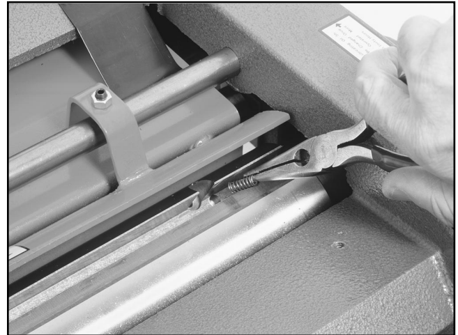
Figure 14. Placing springs into knife slots.
