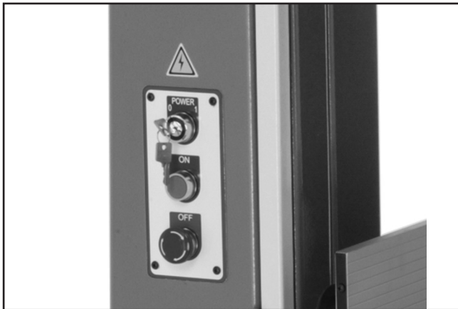
Figure 8. G0513X2 switch disabling key and ON/OFF switch.
