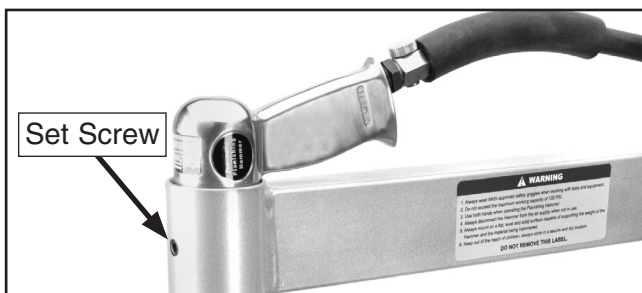
Figure 7. Hammer installed in C-frame.
