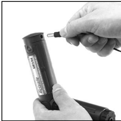
Fig 2. Plugging charger into battery.
