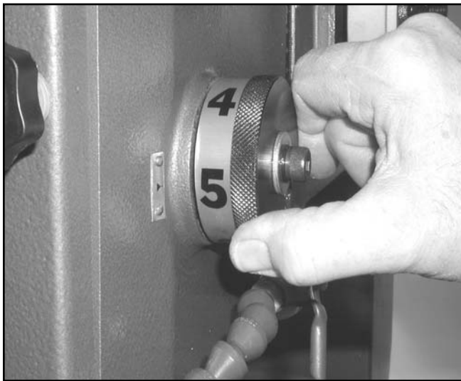
Figure 19. Depth control ring.
