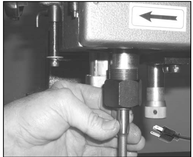
Figure 8. Installing the router bit.
