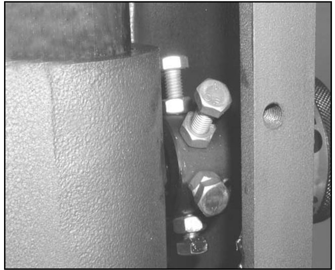
Figure 20. Locking bolts and lock nuts.
