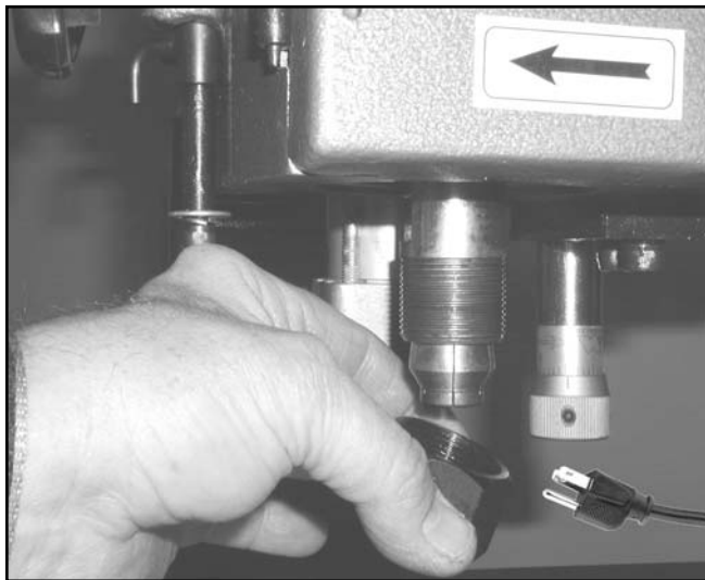
Figure 7. Installing collet nut.
