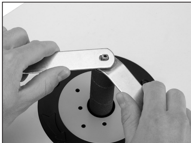
Figure 8. Loosening the spindle hex nut.
