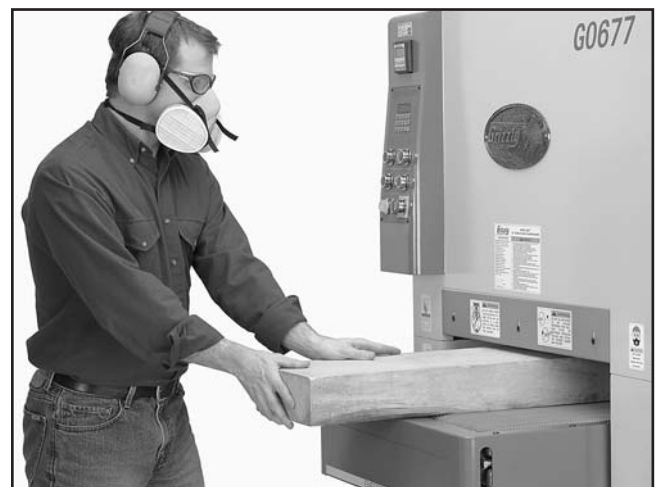
Figure 33. Operator feeding workpiece at correct body position and out of the way of potential kickback.
