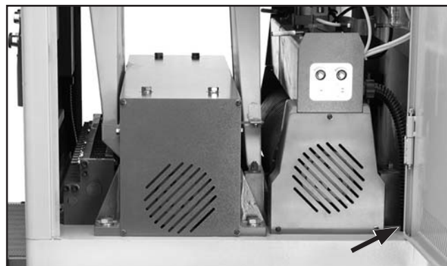
Figure 60. Right rear table-frame height check location.
