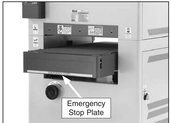
Figure 32. Emergency stop plate.
