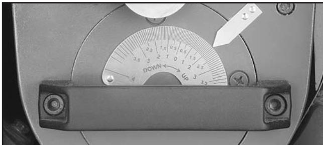
Figure 34. Spiral cutterhead raised to 2mm position on height scale.
