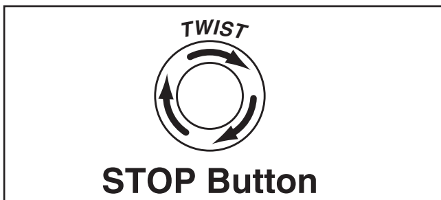
Figure 15. Resetting the STOP button.
