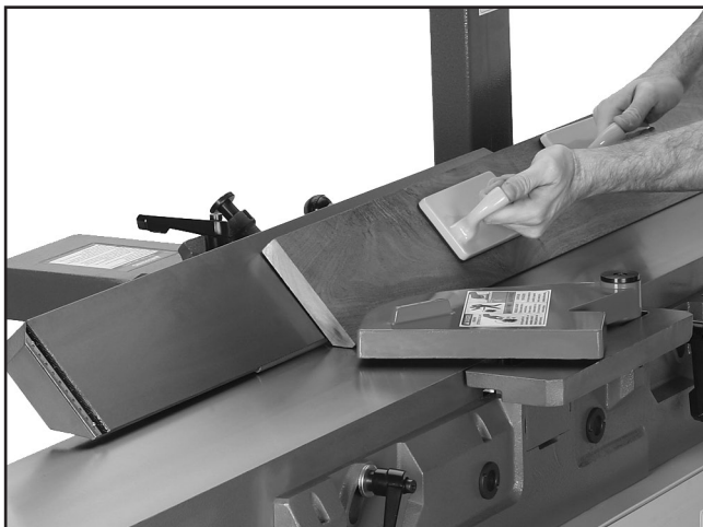
Figure 32. Typical bevel cutting operation, fence stop at 45° outward.
