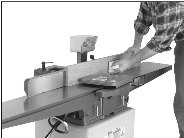
Figure 30. Typical edge jointing operation.
