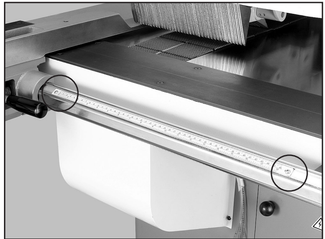
Figure 15. Phillips head screws securing the fence scale.
