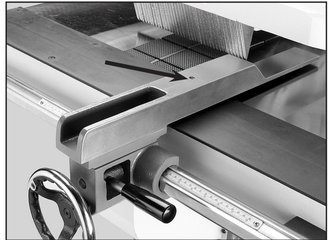
Figure 31. Fence ride height adjustment.
