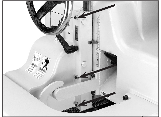
Figure 33. Gib adjustment setscrews.
