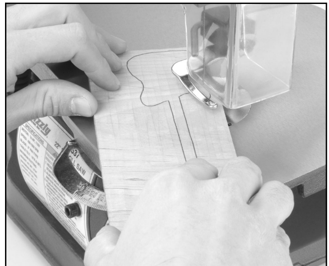
Figure 13. Making a curved cut.
