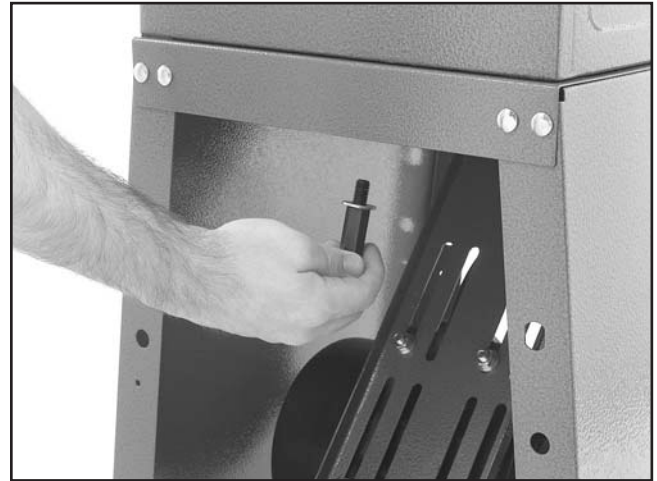
Figure 16. Installing special hex bolt.
