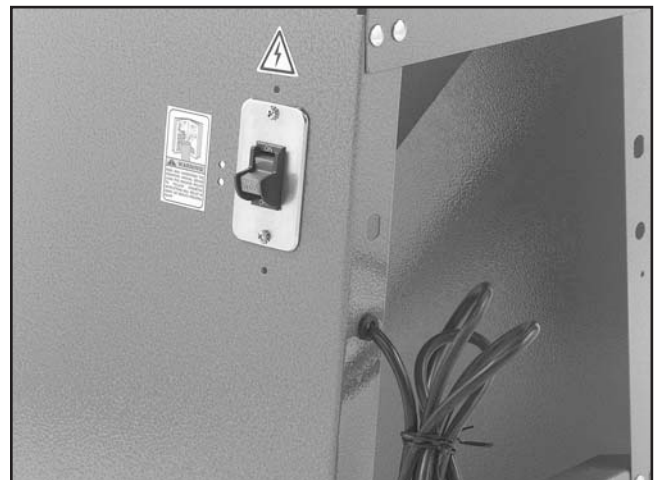
Figure 12. Switch & cord installed on stand.
