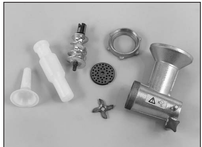
Figure 40. Meat grinder components disassembled for cleaning.
