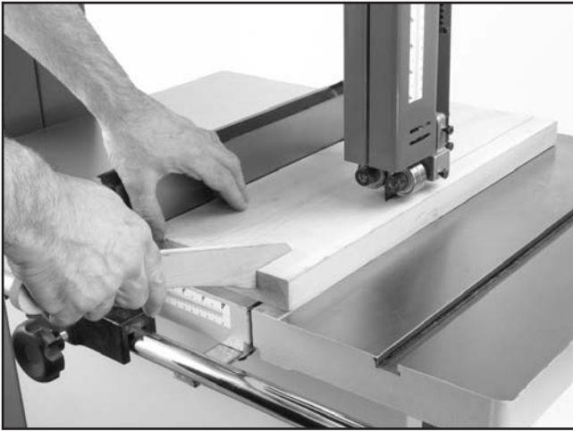
Figure 30. Ripping with a push stick.
