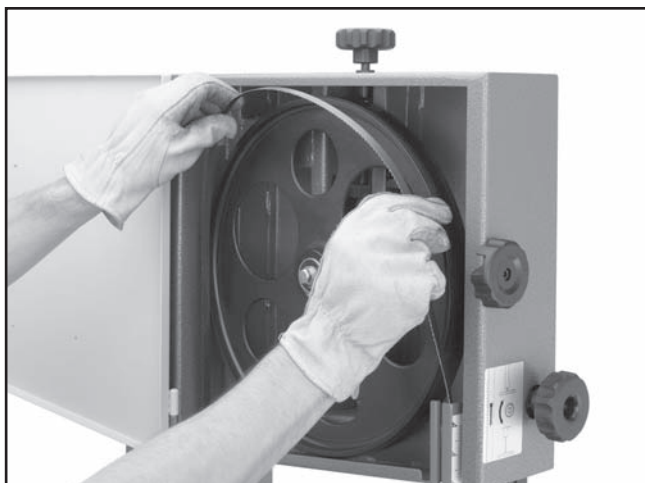
Figure 36. Placing blade on the wheels.
