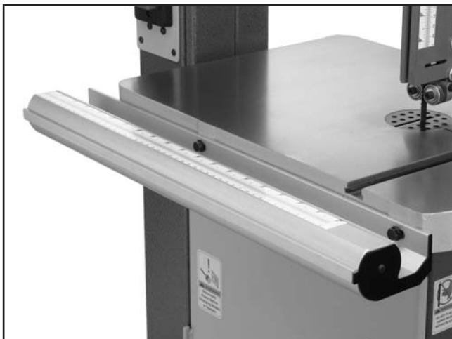
Figure 12. Installed fixed rail.
