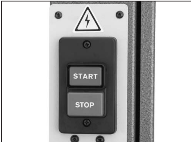
Figure 27. G0570 START/STOP switch.
