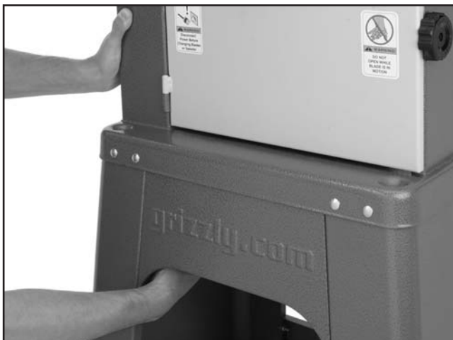
Figure 10. Securing the body to the stand.
