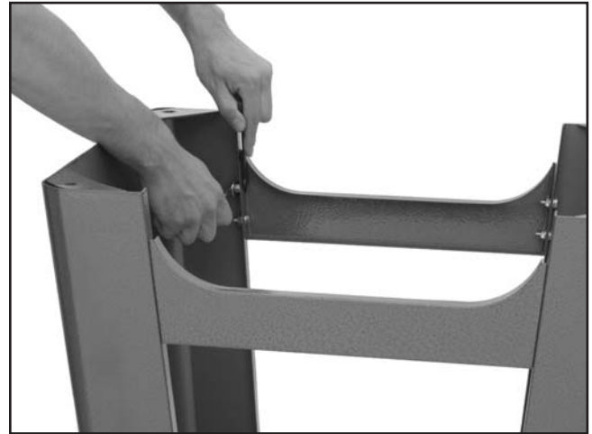
Figure 8. Lower side covers bolted to stands.
