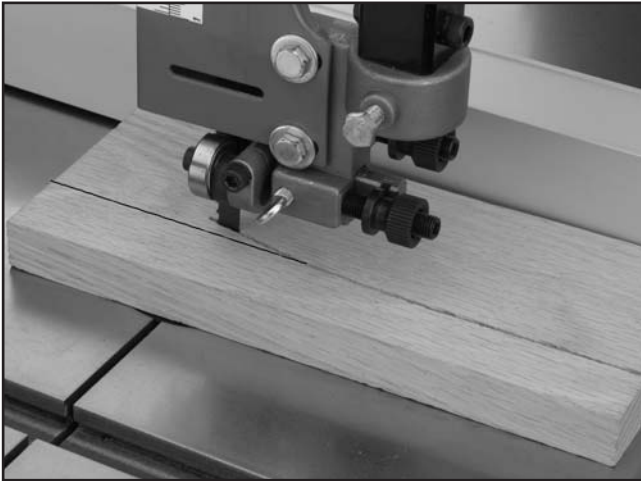
Figure 29. Blade leading away from line of cut.
