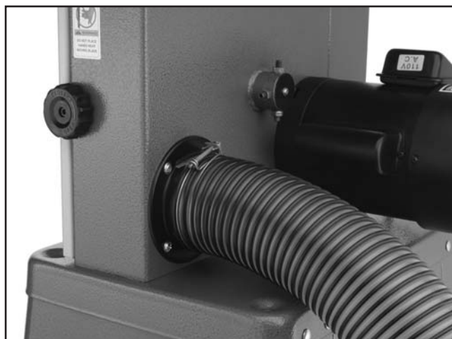
Figure 14. Dust hose attached to dust port.
