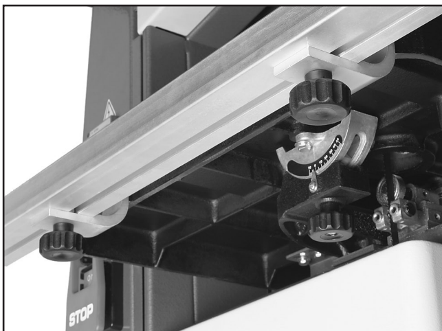
Figure 10. Fastening front fence rail.
