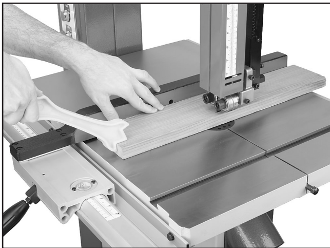
Figure 32. Typical ripping operation.
