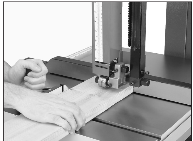
Figure 33. Typical crosscutting operation.
