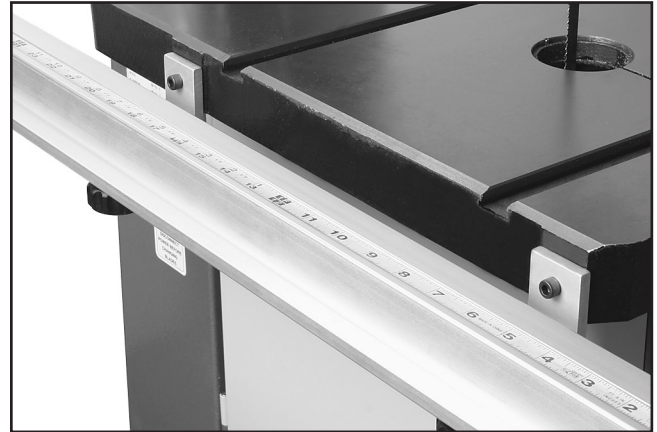
Figure 15. Scale installed on front fence rail.
