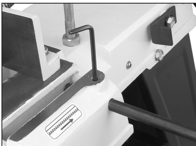
Figure 14. Installing work stop shaft.
