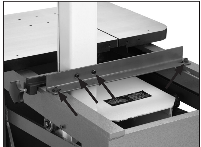
Figure 8. Removing shipping bracket.
