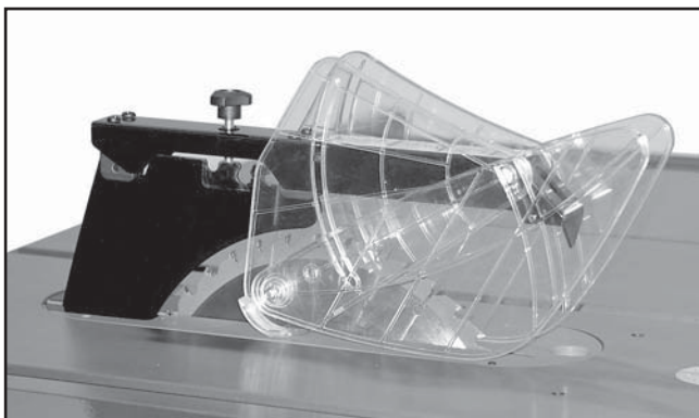
Figure 52. Guard installed without pawls.
