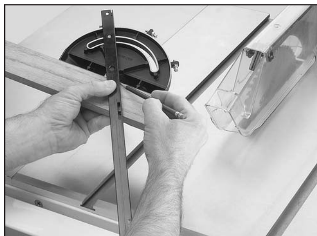
Figure 61. Example of marking miter line.
