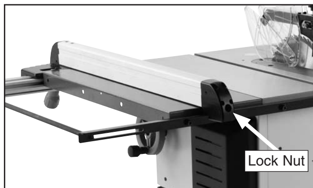
Figure 121. Location of lock nut for adjusting clamping pressure.
