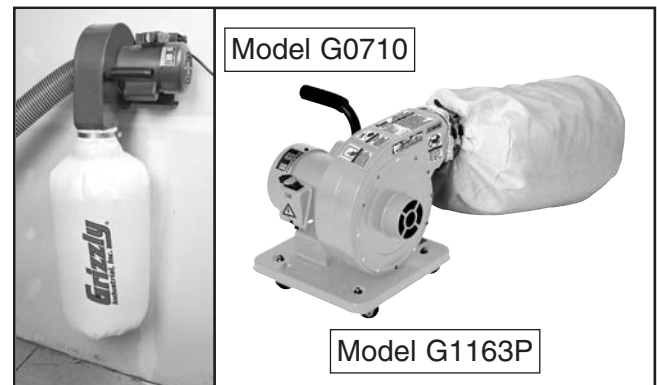
Figure 102. Point-of-use dust collectors.
