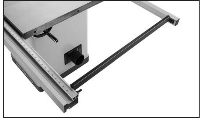
Figure 37. Fence rail brace installed.
