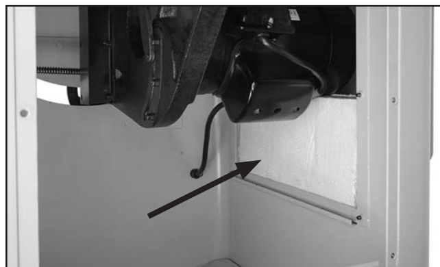
Figure 29. Location of styrofoam block to be removed.
