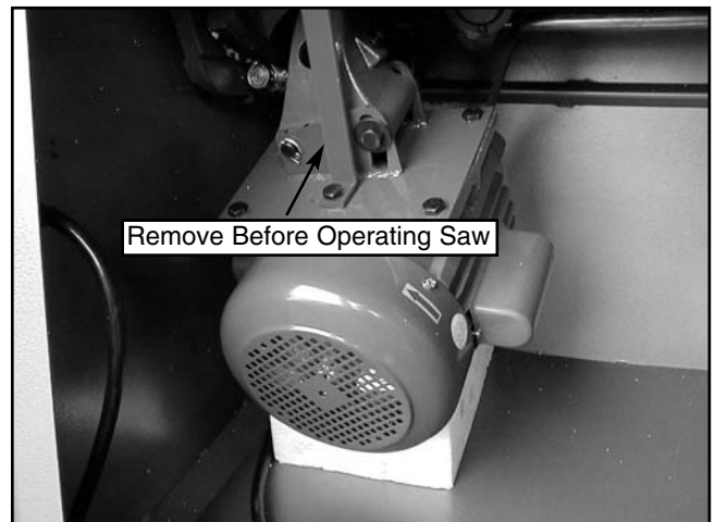
Figure 10C. Remove motor bracket.
