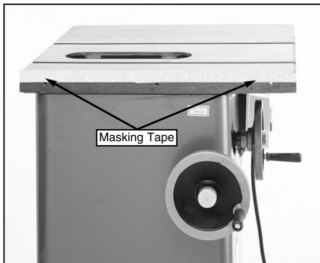
Figure 7. Using tape to shim for wing alignment.
