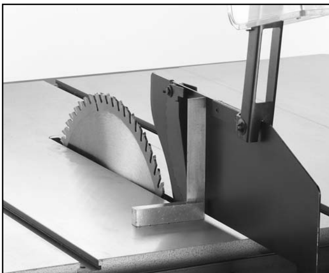
Figure 13. Guard assembly square to table.
