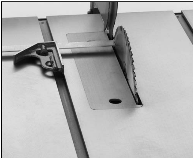
Figure 21. Adjusting blade to miter slot.
