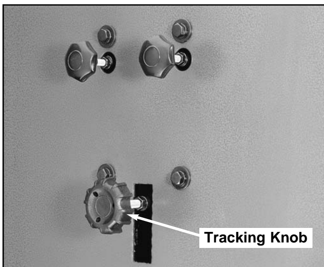
Figure 3. Tracking knob adjustment location.
