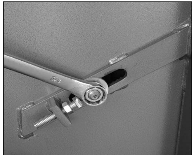
Figure 12. Loosening the adjuster nut.
