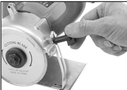
Figure 6. Adjusting the cutting depth.
