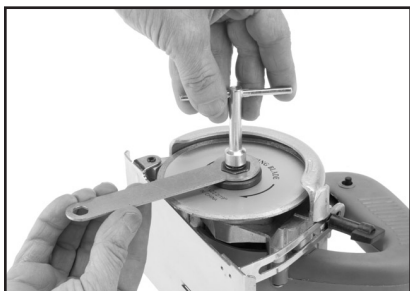
Figure 7. Replacing the diamond blade.
