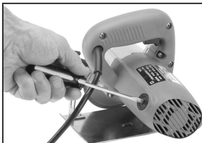
Figure 8. Removing a brush cap.
