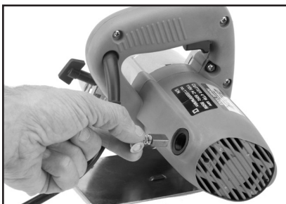
Figure 9. Replacing a motor brush.
