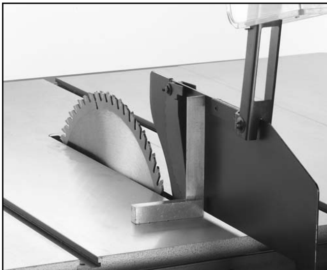
Figure 13. Guard assembly square to table.
