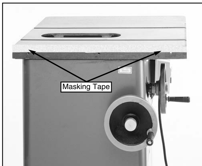
Figure 7. Using tape to shim for wing alignment.
