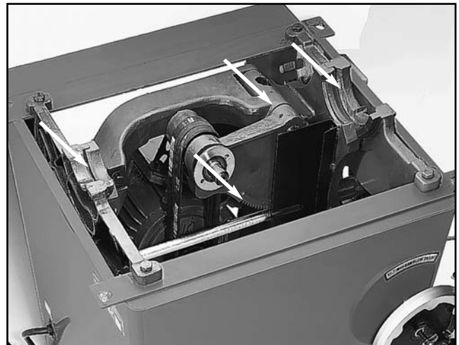
Figure 43. Lubricate these areas.
