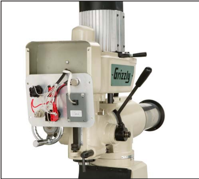
Figure 68. Control panel wiring.
