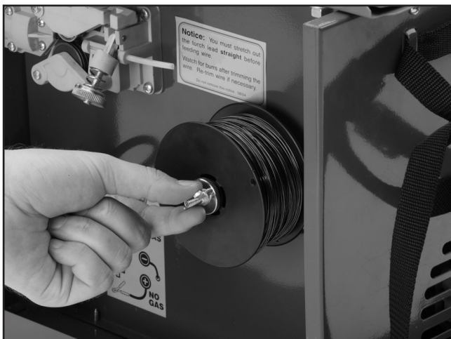
Figure 6. Replacing the wire spool.
