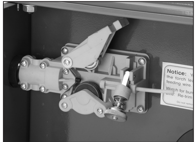
Figure 7. The open wire feed mechanism.
