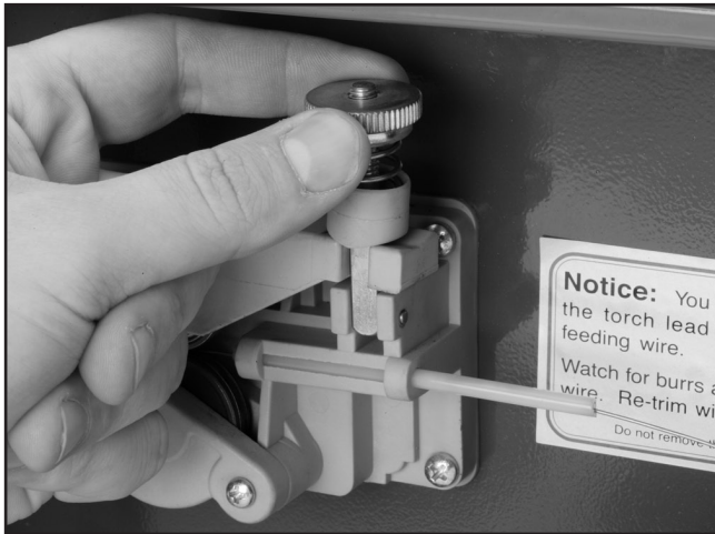
Figure 9. Adjusting the feed tension.
