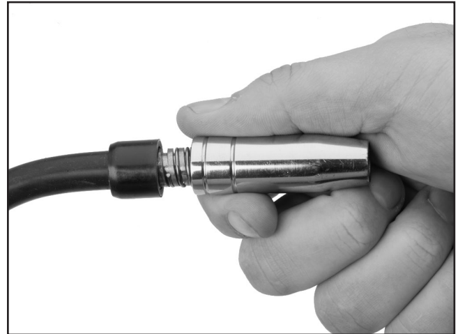
Figure 10. Removing the welding torch nozzle.
