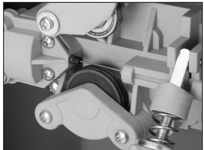
Figure 8. Feeding the wire.
