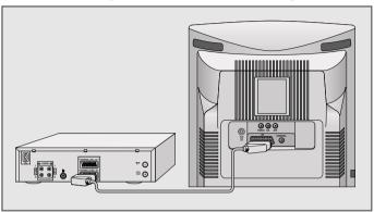
Connect the »AV1« socket on the television to the corresponding socket of the video recorder or set-top box using a Euro-AV (Scart) cable.
