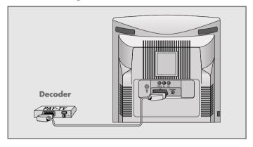
1 Connect the »AV1« socket on the television set and the corresponding socket on the decoder using a EURO-AV cable.
