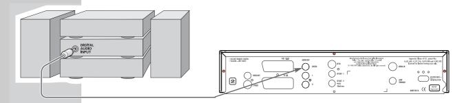
1 Plug a standard phono cable into the »DIGITAL AUDIO OUT« sockets on the receiver-player and into the appropriate sockets on the HiFi system.
