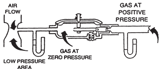
Figure 2.16 – LP Gas Carburetion Diagram
