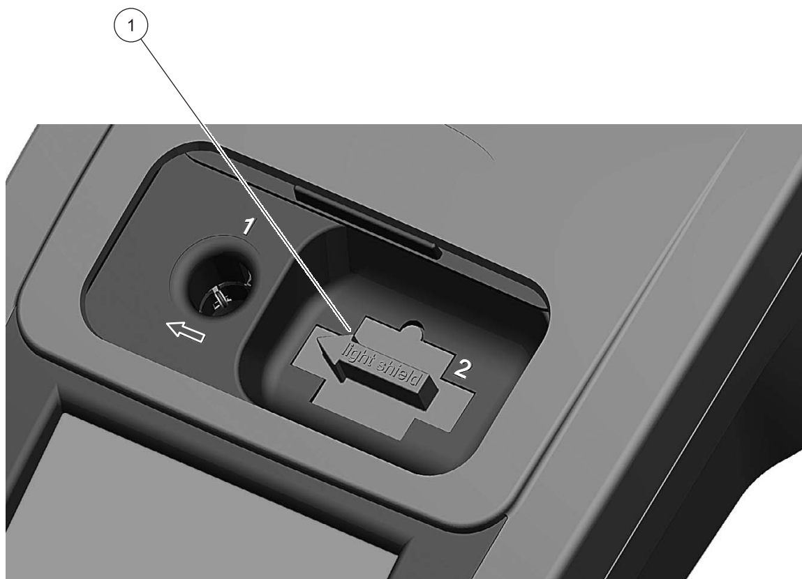
Figure 7 Light Shield in place
